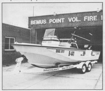
The Port (left) side has a 34" cutout for the ease of sliding in a back boarded patient at water level instead of over the gunwale.
